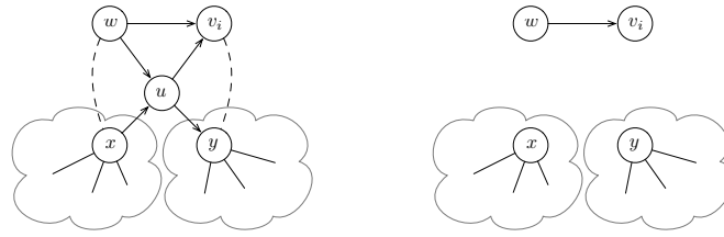
Figure 3: Impact of false positive and false negative edges on connected components discovery when using transitive closure. Left: vertex v_i is added to the graph with single component consisting of vertices \{w, u, x, y\} . We consider two cases where edges (w, x) and (v_i, y) are incorrectly missing, or edges (x, u) and (u, y) are incorrectly introduced. Right: After performing transitive closure on u , in both cases the graph will consist of three connected components instead of one component.
