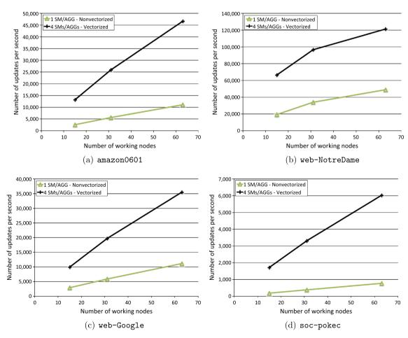
Fig. 12. co-BFS: the performance is expressed in the number of updates per second. The best worker-node configuration, "8 threads, 1 graph/NUMA", is used for the experiments.
