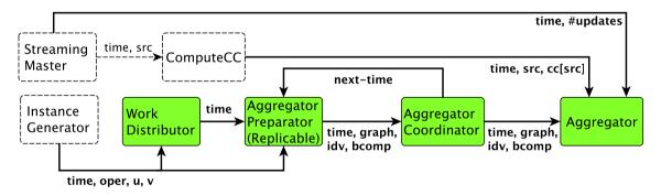
**Fig. 8.** Replicating Aggregator for a better scaling when the number of processors is large.
