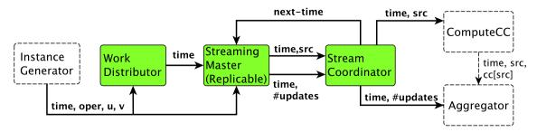
Fig. 7. Replicating StreamingMaster for a better scaling when the number of processors is large.
