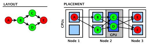
Fig. 4. A toy filter-stream application layout and its placement.
