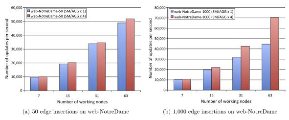
Fig. 11. Parallelizing StreamingMaster and Aggregator: the number of updates per second for web-NotreDame with 50 and 1000 Streaming Events, respectively. The best node configuration from Fig. 9, i.e., 8 threads, 1 graph/NUMA, is used for both cases.
