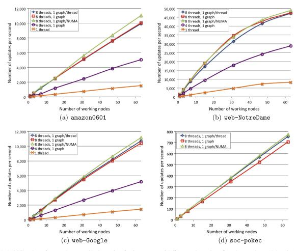
**Fig. 9.** Scalability: the performance is expressed in the number of updates per second. Different worker-node configurations are shown. "8 threads, 1 graph/ thread" means that 8 *ComputeCC* filters are used per node. "8 threads, 1 graph" means that 1 *Preparator* and 8 *Executor* filters are used per node. "8 threads, 1 graph/NUMA" means that 2 *Preparators* per node (one per NUMA domain) and 8 *Executors* are used.
