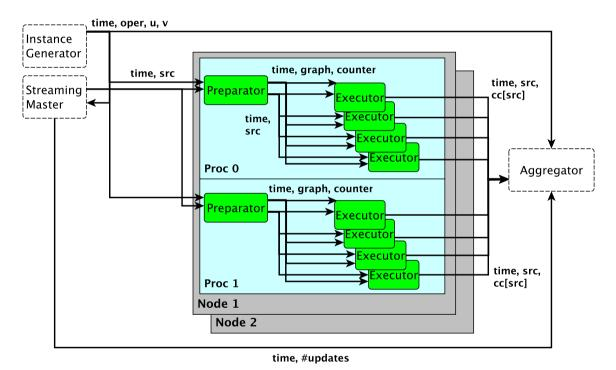
Fig. 6. Placement of Streamer using 2 worker nodes with 2 quad-core processors. (The node 2 is hidden). The remaining filters are on node 0.
