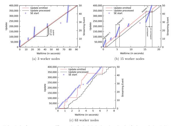
Fig. 10. Execution logs for web-NotreDame on different number of nodes. Each plot shows the total number of updates sent by StreamingMaster and processed by the Executors, respectively (the two lines), and the times at which StreamingMaster starts to process Streaming Events (the set of ticks).
